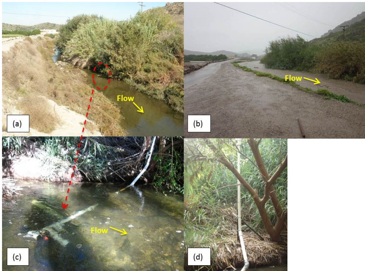
Figure 3. Sensor system at 9A_HOWAR: (a) Conejo Creek looking upstream near Howard Road toward Camarillo WRP; (b) March 20, 2011 storm flow looking upstream from similar location; (c) Sensors staked and supported in channel in PVC conduit; (d) Electronics housing staked on river bank.
