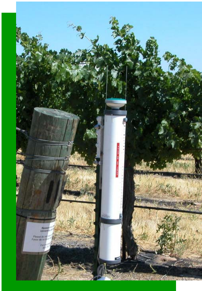
Figure 1. An atmometer installed on a steel fencepost at the end of a vineyard row.
